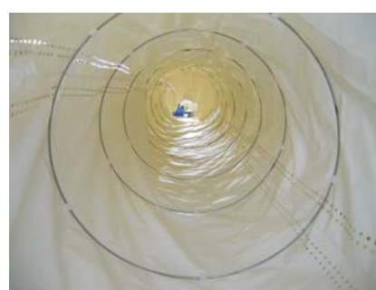
4. Internal part of diffuser with reinforcement rings
